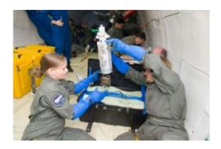
Graduate student Laura Jones and master of engineering student William Wilson demonstrate flux pinning of a prototype CubeSat to a superconductor while aboard NASA's microgravity aircraft, Aug. 10.
