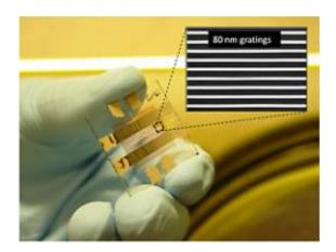
A researcher holds a sample of prototyped solar cells. The inset is an electron micrograph of the nanostructures.
