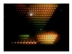
Pictured are nano dipole antennas under a microscope. The colors reflect the different transmission frequencies. Credit: LTI
