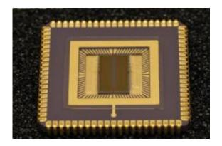
The innovative CMOS image sensor can distinguish color and is much more lightsensitive than conventional sensors. Credit: Fraunhofer IMS
