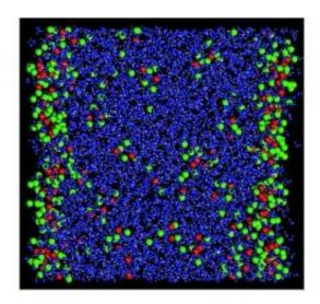
Snapshot from the simulations with the polarizable potential. Water molecules are in blue. The Cl- ions are in green and the corresponding Sr2+ ions are in red.
