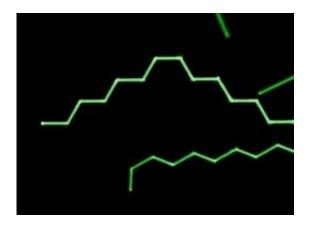
This is a false-color scanning electron microscope image of the zigzag nanowires in which the straight sections are separated by triangular joints and specific device functions are precisely localized at the kinked junctions in the nanowires. Credit: Bozhi Tian, Lieber Group, Harvard University
