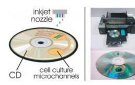
Scientists have used an Epson R280 inkjet printer to dynamically control gene expression in two dimensions. Image credit: Cohen, et al.
