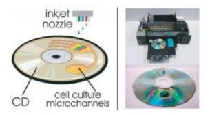
Scientists have used an Epson R280 inkjet printer to dynamically control gene expression in two dimensions. Image credit: Cohen, et al.
