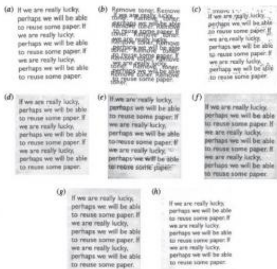
Reprinted office paper. (a) For comparison: text on fresh paper, (b) water, (c) dimethylsulphoxide, (d) chloroform, (e) dichloromethane, (f) acetone, (g) 80% acetone + 20% chloroform (h) 40% chloroform + 60% dimethylsulphoxide. Image copyright: Counsell and Allwood.
