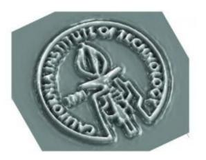
This is a simulation of Caltech logo formed in a 100 nm polymer film by thermocapillary patterning. Credit: Dietzel and Troian/Caltech
