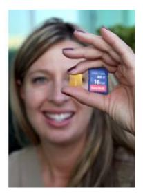
SanDisk announced it has begun production shipments of flash memory cards based on the company's advanced X4 flash memory technology. This innovative new technology holds four bits of data in each memory cell, twice as many as the cells in conventional multi-level cell (MLC) NAND (2-bits-per-cell) memory chips.
