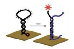
A new ultrafast DNA sensor contains hairpin-shaped DNA strands attached to a gold film. The DNA unfolds when it captures the target gene sequence, and an attached fluorescent molecule glows.
