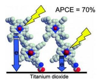
Photoexcited porphyrin dimers incorporated into thin dye-sensitized solar cells show efficient and fast electron injection, improving the light harvesting efficiency by 30%. Image copyright: Mozer, et al.
