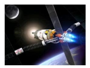
In the VASIMR rocket, magnetic fields force the charged plasma out the back of the engine, producing thrust in the opposite direction. Image copyright: Ad Astra Rocket Company.
