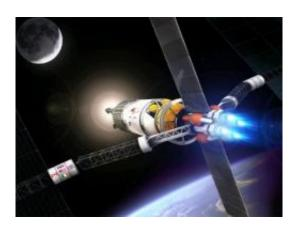
In the VASIMR rocket, magnetic fields force the charged plasma out the back of the engine, producing thrust in the opposite direction. Image copyright: Ad Astra Rocket Company.
