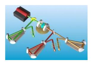
Scientists have entangled light of three different colors. In the set-up, the optical parametric oscillator (center) is pumped by a coherent light source, producing three light fields of different wavelengths (green, red, and orange arrows). Entanglement is verified using an analysis cavity for each beam, and the golden rings illustrate the tripartite entanglement among the optical fields. Image copyright: A.S. Coelho, et al. Reprinted with permission from AAAS.
