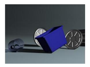
Whether metal or plastic, objects made up of thin shells have a characteristic way of making noise that can be simulated by a computer to synthesize sound for animated films and virtual reality. Image: James Lab/Cornell University
