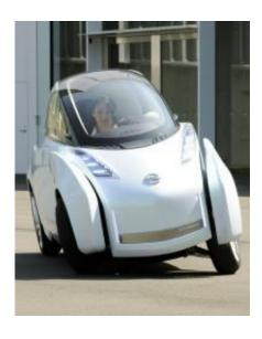
An employee of Japan's auto giant Nissan demonstrates the new concept vehicle, the "Land Glider", a tandem-ride ultra light-weight electric vehicle with a narrow body at the company's design center at Atsugi city in Kanagawa prefecture, suburban Tokyo. The car shifts its centre of gravity whilst turning by leaning like a motorcycle.
