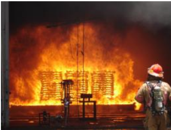
Well deck fire suppression tests
