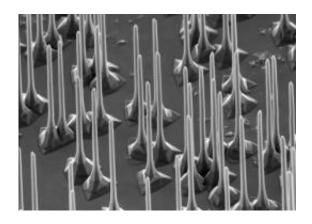
Scanning electron microscope of nanowires ready for device assembly using optical tweezers. Image courtesy of Dr H. Tan at ANU
