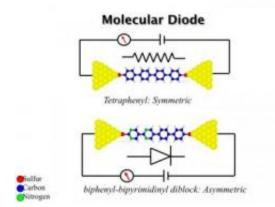
This is a schematic for molecular diode. The symmetric molecule (top) allows for two-way current. The asymmetrical molecule (bottom) permits current in one direction only and acts as a single-molecule diode. Credit: Biodesign Institute at Arizona State University
