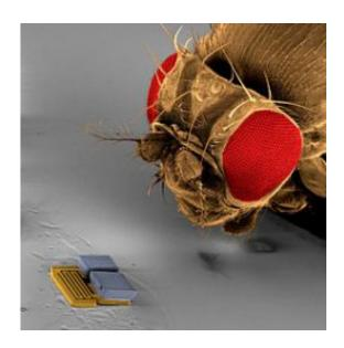
A microrobot used at the RoboCup 2009 nanosoccer competition by the team from Switzerland's ETH Zurich is compared in size to the head of a fruit fly. The robot, which is operated under a microscope, is 300 micrometers in length or slightly larger than a dust mite. Credit: ETH Zurich
