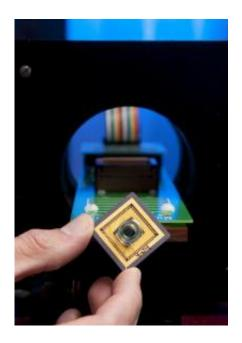
The magnetonanosensor has 64 sensors capable of detecting up to 64 different proteins. In the center of the chip is the well that holds the fluid of interest. The reader that measures the magnetic fields of the sensors is in the background. Thumb and fingers are courtesy of Richard Gaster, M.D./Ph.D. candidate in both bioengineering and the school of medicine. Credit: Linda Cicero, Stanford News Service
