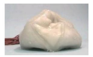
The blob bot uses a jamming mechanism to change its shape and roll, enabling it to squeeze into small spaces. Credit: iRobot.
