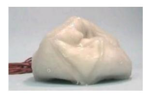
The blob bot uses a jamming mechanism to change its shape and roll, enabling it to squeeze into small spaces. Credit: iRobot.
