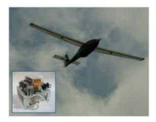
This photo shows the Ion Tiger in flight. The 550-watt fuel cell is show in the box in the lower left corner. Credit: Naval Research Laboratory
