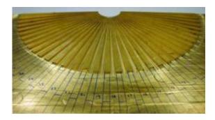
The acoustic hyperlens is fashioned from 36 brass fins arranged in the shape of a hand-held fan. Each fin is approximately 20 centimeters long and three millimeters thick. Credit: Courtesy of Xiang Zhang research group
