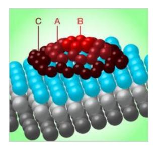
Carbon atoms form dome structures on iridium substrates, en route to forming larger scale graphene sheets. Credit: Image courtesy of Alan Stonebraker.
