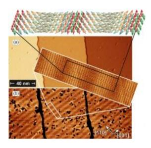
(Top) Schematic of the spin structure of the Mn monolayer on W(110) (6-nm repeat structure). (a) Topography and (b) differential conductance at 40 K. (Inset) High-resolution topographic data taken with a spin-sensitive tip; stripe contrast is related to the degree of antiferromagnetic order.
