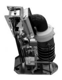
The equipment removes fine dust particles effectively from product surfaces -- and collects them safely. Credit: Fraunhofer IGB
