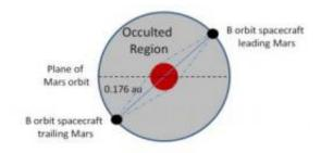
This is an end-on view of an alternative Mars/Earth communication relay architecture option, looking into the Ecliptic plane. Credit: Credits: ESA/University Strathclyde/University Glasgow
