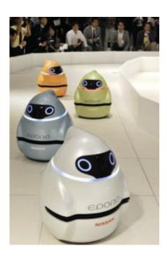
Robot cars designed by Nissan travel in group and move to avoid obstacles at a press preview at the company's headquarters in Yokohama, suburban Tokyo. With these robots, engineers in Japan say they are a step closer to developing technology they hope will cut the risk of car crashes -- by mimicking the behaviour of fish.
