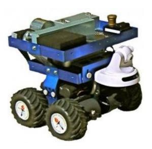
The CYCLOPS mobile robotic platform is designed to be used as a surrogate for blind persons in the testing of visual prostheses. Credit: Caltech/Wolfgang Fink, Mark Tarbell
