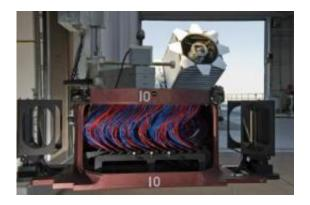
This is one of the BOSS fiber cartridges, containing 1,000 optical fibers that guide light from a "plug plate" targeting specific galaxies and quasars to the spectrograph; Sloan Foundation telescope is in the background. Credit: Dan Long, Senior Operations Engineer, Apache Point Observatory
