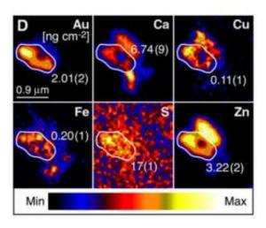
This image shows maps of pure gold with other elements. By determining what elements there are, scientists can see where the gold is located in relation to the cells. These maps are quantitative X-ray fluorescence maps showing the distribution of gold, calcium, copper, iron, sulfur and zinc in an individual cell after a minute exposure to Au(III) at pH 7.0 (the quantified area is marked in the image, and concentrations are in the image). Credit: Reith et al, PNAS 5-9 October 2009.
