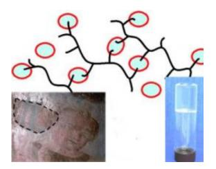
Oil-in-water nanocontainers within an aqueous polymer network were effective for the low-impact selective cleaning of painted and gilded surfaces. Interactions with the polymer (black in the schematic illustration) did not alter the structure of the microemulsion nanodroplets (light blue and red) significantly. A photograph of an equilibrated mixture of the microemulsion and the polymer is shown. Credit: (C) Wiley-VCH 2009
