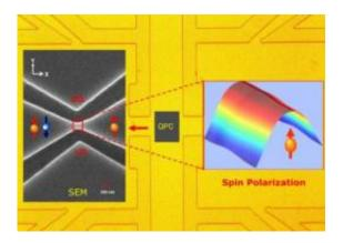
(Left) Scanning electron micrograph of the quantum point contact schematically illustrates unpolarized (spin up and spin down) electrons incident on the left coming out of the device spin-polarized with spin up. (Right) Spatial distribution of spin polarization in the quantum point contact constriction. Credit: Illustration by Professor Philippe Debray, University of Cincinnati
