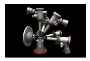
The main experimental chamber of the AMO instrument, the high-field physics end-station. Here, a gas jet sends pulses of sample gas into the chamber where it will be ionized by X-rays from the LCLS. The results are detected by several spectrometers arrayed around the central interaction region. Read more in the AMO Technical Specifications. (Image: SLAC Infomedia Solutions.)
