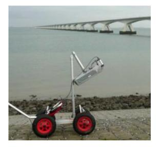
Miramap's instrument can be mounted on a cart and walked across a dam or dike to measure very accurately the underground soil moisture levels. Credits: Miramap
