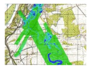
Soil moisture map of a Danube river section in dry conditions. The colours correspond to the soil moisture gradations in the upper 0-5 cm-thick layer. Dark green ranges between 0 and 0.05 m3/m3 Light green ranges between 0.05 and 0.10 m3/m3 Light blue ranges between 0.10 and 0.20 m3/m3 Dark blue ranges between 0.20 and 0.35 m3/m3, and represents open water. Credits: Miramap
