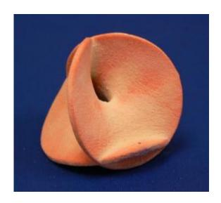
This is an object printed from powdered glass, using the Solheim Lab's new Vitraglyphic process. Credit: University of Washington
