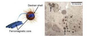
An iron-centered nanoparticle (left) analyzed at NIST's Center for Neutron Research has a coating of the sugar dextran, whose tendrils prevent groups of the particles from clumping. When tumor cells ingest them (right), the particles still congregate closely enough to share heat when stimulated by a magnetic field, killing the cells. White arrow indicates a red blood cell. Credit: (l.) J. Aarons; (r.) A. Guistini, R. Strawbridge and P. Hoopes, Dartmouth College
