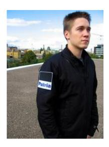
Through the ESA Advanced Research in Telecommunications Systems (ARTES) 5 project 'Textile Antennas', the Finnish Patria Aviation Oy company has demonstrated that an antenna can be built using textiles that can be worn and used for personal satellite communication. The antenna is here seen attached to the sleeve of a jacket. Credits: Patria Aviation Oy
