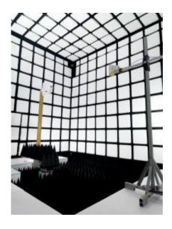
This is the NPL Smart Chamber with Orbit roll over as positioner. Credit: NPL
