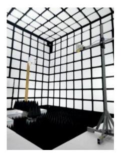
This is the NPL Smart Chamber with Orbit roll over as positioner. Credit: NPL
