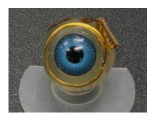
A model of the retinal implant: The coil that surrounds the iris receives visual data from a camera mounted on a pair of glasses. The coil sends the images to a chip attached to the side of the eyeball, which processes the data and sends it to electrodes implanted below the retina. Photo - Courtesy Shawn Kelly
