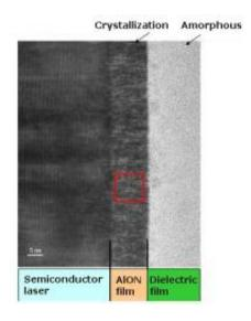
A cross-sectional image of the semiconductor laser with an aluminum oxynitride film.
