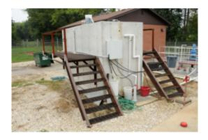
This pilot-scale testing unit demonstrates how the wastewater treatment system would work. Recently Wang received approval for full-scale system demonstration.
