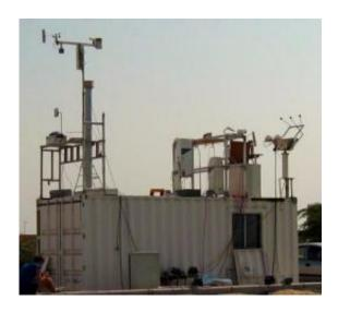
This facility, known as MAARCO, is a transportable climate-controlled laboratory containing scientific instrumentation for measuring atmospheric aerosols, trace gases, chemistry, radiative properties, cloud structure and meteorology. Credit: Naval Research Laboratory
