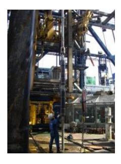
This image shows a worker lowering the tool to measure stress and pore fluid pressure in the subsurface. Credit: Copyright: JAMSTEC/IODP
