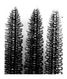
Ames Laboratory senior metallurgist Rohit Trivedi will be studying how crystals, such as these nickel-based superconductors, grow in low gravity experiments on board the International Space Station. Credit: USDOE's Ames Laboratory
