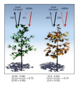
NDVI is calculated from the visible and near-infrared light reflected by vegetation. Healthy vegetation (left) absorbs most of the visible light that hits it, and reflects a large portion of the near-infrared light. Unhealthy or sparse vegetation (right) reflects more visible light and less near-infrared light, yielding a lower NDVI. Credit: Robert Simmon
