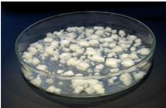
A synthetic salt crust obtained from artificial sea salt and an alpha-amino acid.
