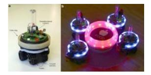
(A) The robot used for the experiments, which has floor sensors to distinguish food and poison sources, and a ring of blue lights. (B) Robots emitting blue light near a food source. Image copyright: Sara Mitri, et al.
