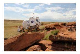
LER, the next-generation rover, an all-electric vehicle with 12 wheels, is shown here crawling over the rough terrain of Black Point Lava Flow. Credit: NASA
